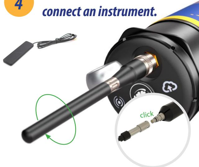
After connecting the external or on-board antenna and instrument, follow the instructions on the next pages of this quickstart guide.
