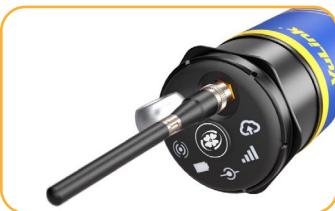
Make sure the antenna is properly attached before proceeding.
