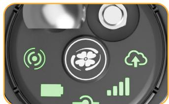
Press the button. All LEDs turn on. Each LED changes color according to device status.
