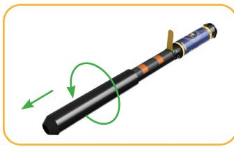
Remove the battery cover by twisting it counter-clockwise and pulling down.
