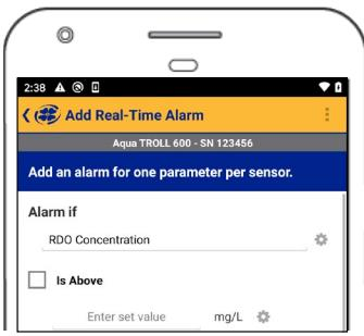
Select the parameter that should trigger the alarm and set the limits.
