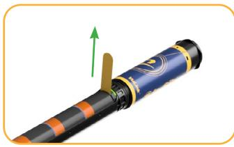
Remove the yellow tab to allow current to flow through the batteries. Replace the cover.
